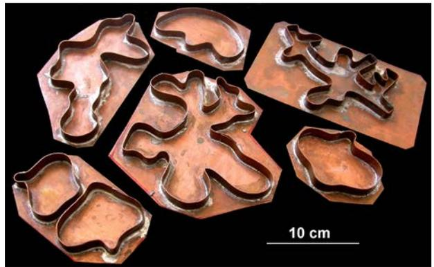
Fig. 2: The ice molds can be made in a wide range of sizes and shapes. These may be based on the natural chamber shapes (as shown here), or deviate from the natural shapes to suit the conditions of experiments.
