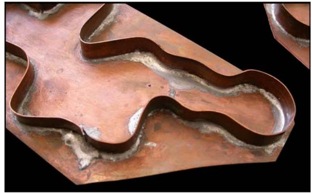
Fig. 1: Close up view of an ice mold showing the water tight solder joint.
