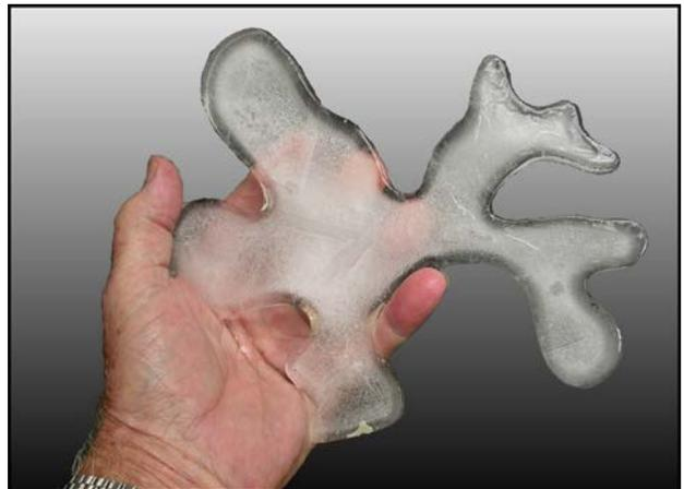
Fig. 3: An ice chamber freed from its mold. This chamber should be cooled with dry ice before planting in the soil.
