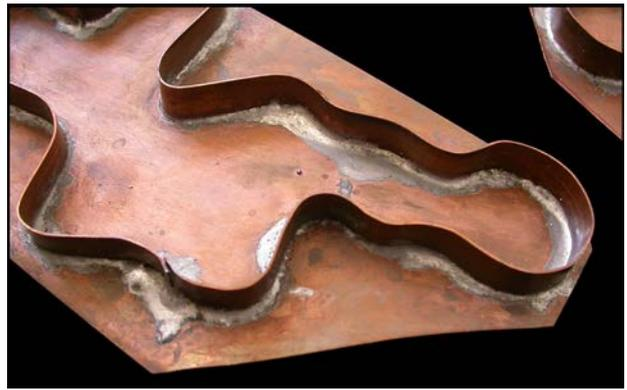
Fig. 1: Close up view of an ice mold showing the water tight solder joint.
