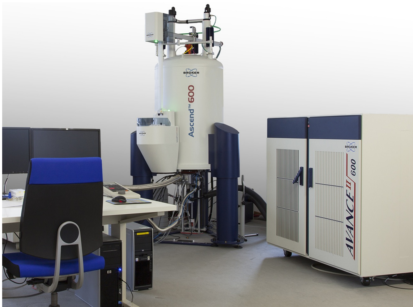
FIG. 1. Picture of a mid-range NMR spectrometer (Courtesy of Bruker-Fällanden). It is composed of a cryomagnet ( center ), an electronic console ( right ) and the user console ( left ). The strength of the magnet is graded according to the frequency of the ^1\text{H} NMR signals (here ^1\text{H} = 600\text{ MHz} or B_0 = 14\text{T} ). The magnet Dewar contains the superconducting coil (not visible) at liquid helium temperature and a detection probe, which is also cooled at 15–20K to minimize the thermal noise (cryoprobe). The sample is inserted from the top of the bore by means of a pneumatic lift. The r.f. pulse and pulsed field gradients enter the probe from the bottom of the magnet bore and two insulated pipes provide the cooling for the cryoprobe and the temperature regulation of the sample (–20 to 80 °C). Most recent magnets are actively shielded, i.e. the stray field outside the magnet itself is minimized. The electronic console contains a pulse programmer that generates and amplifies r.f. and pulse field gradient pulses sent to the probe and trigger the data acquisition: modern spectrometers are equipped with four channels (usually ^1\text{H} , ^{13}\text{C} , ^{15}\text{N} , and ^2\text{H} for the frequency-field lock) with independent frequency synthesis and amplification. Although the list price of NMR spectrometers has considerably dropped over the years, it does not depend linearly with the magnetic field. The price ratio for 600, 800, and 950 MHz is roughly 1: 2: 6.
