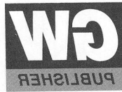
2. Static pattern on drum. Dark areas are negative or no charge. White areas are positive charge.
