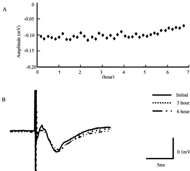
Fig. 4. Stability of fEPSP. (A) Measurements of fEPSP amplitude with time. Schaffer collateral axons in region CA3 were stimulated by a pair of microelectrodes with biphasic constant current pulses (amplitude,  $\pm 18 \mu\text{A}$ , duration,  $100 \mu\text{s}$ ), and fEPSPs were recorded at the stratum radiatum in CA1 for 7 h. The slice was perfused at 2 ml/min with oxygenated recording buffer at  $34^\circ\text{C}$ . (B) Comparison of raw waveforms recorded at channel 7 at 0, 3, and 6 h.
