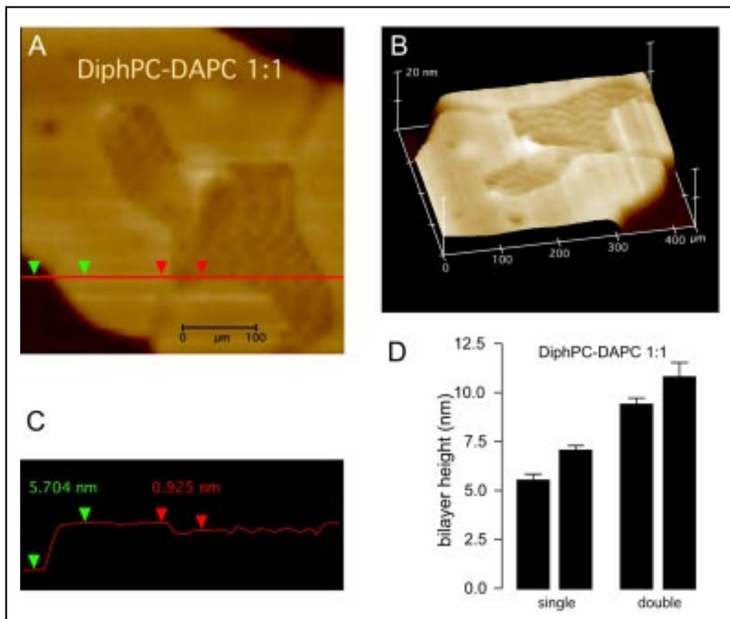
bilayers. The left two bars (single) and right two bars (double) represent the thicknesses of single and double bilayers, respectively. As evident, two discrete heights can be measured in both single and
